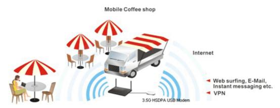
After connecting into the router, 3G USB Modem will be regarded as the fifth WAN port. However, the other Ethernet WAN ports still can be used and Load-Balance can be done in the router. Besides, 3G USB Modem also can be used as backup device. Therefore, when other Ethernet WAN ports are not available, the router will use 3.5G for supporting automatically. The supported 3G USB Modem will be listed on DrayTek web site. Please visit www.DrayTek.com for more detailed information.
