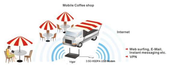
After connecting into the router, 3G USB Modem will be regarded as the fifth WAN port. However, the other Ethernet WAN ports still can be used and Load-Balance can be done in the router. Besides, 3G USB Modem in WAN5 also can be used as backup device. Therefore, when other Ethernet WAN port is not available, the router will use 3.5G for supporting
