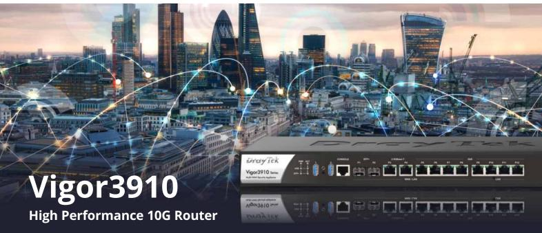
Vigor3910 is capable for bandwidth demanding network. The router features a powerful quad-core processor, six WAN interfaces, including one 10G SFP+ for fiber connectivity, one 2.5G Ethernet, RJ-45, and four Gigabit Ethernet, RJ-45, gives you NAT throughput up to 8.5 Gbps. In addition, the router has four Gigabit Ethernet, RJ-45 as a LAN interface.
