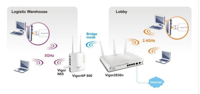
Note: Wireless performance always depends on your specific environment. If your N65 connected to VigorAP 800, the WMM functionality is only working within 2.4GHz frequency.
